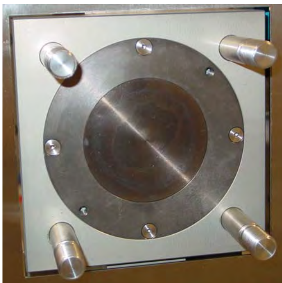
Extruder plate dismantled
